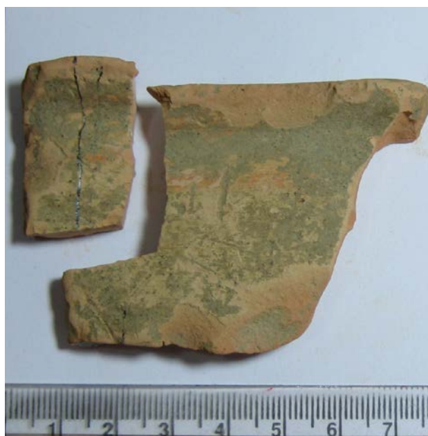
Figure 4. Sample prepared for thin sectioning; a piece of less than 3x3cm is cut from the sherd: a Late Bronze Age Mycenaean krater fragment from Kamaroti. The line on the smaller piece indicates where the thin section will be taken exactly (the thin sections will be cut at the Fitch Laboratory at the British School at Athens)
