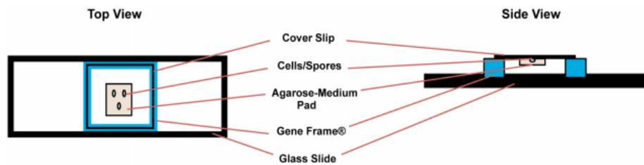
**Figure 1. Closed air-containing chamber for live cell imaging**
